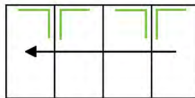
Example 1 Position of glass adjuster kit
