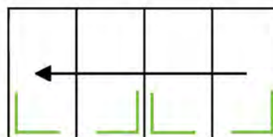
Example 2 Position of glass packers
